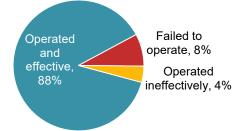
Sprinklers operated in 92% of the fires in which sprinklers were present and the fire was large enough to activate them.
