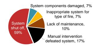
Figure 11. Reasons for sprinkler failures: 2010-2014.
