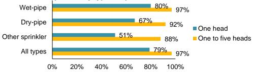
In 97% of the fires in which one sprinkler operated, it was effective. Figure 10 shows that sprinklers were somewhat less likely to have operated effectively when more heads operated.
