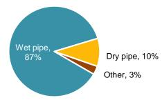
Figure 3 and Table 2 show that dry pipe sprinklers were more common in storage occupancies. "Other" sprinklers were seen most frequently in eating and drinking establishments. It is possible that some of these other sprinklers were actually miscodes of systems designed specifically for cooking equipment.
