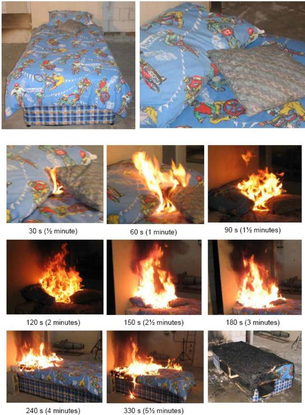
Photographs taken before, during and after bed calorimetry fire
